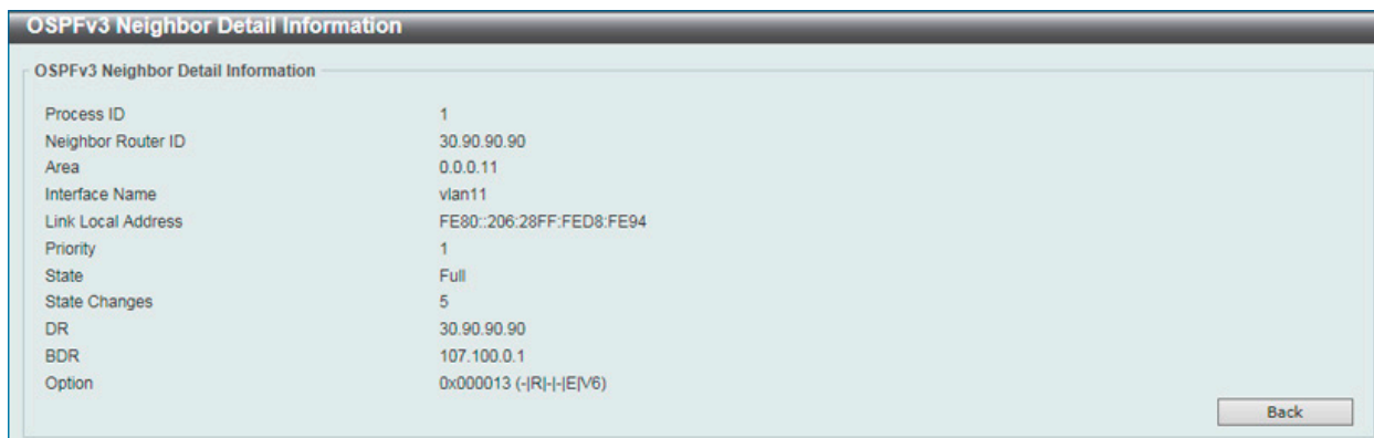
図 9-84 OSPFv3 Neighbor Table (Show Detail) - OSPFv3 Neighbor Detail Information 画面
