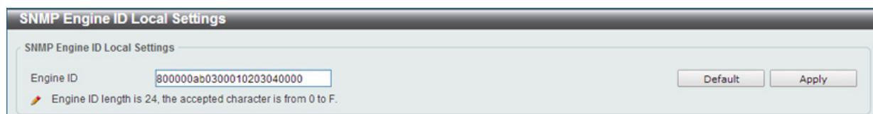
The screenshot shows the 'SNMP Engine ID Local Settings' configuration page. It features a text input field for 'Engine ID' containing the value '800000ab0300010203040000'. Below the input field, a note states: 'Engine ID length is 24, the accepted character is from 0 to F.' To the right of the input field are two buttons: 'Default' and 'Apply'.
