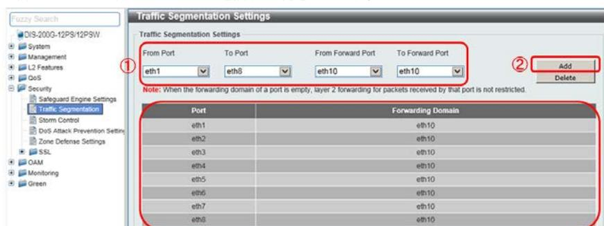
図 16-3 Traffic Segmentation Settings (DIS-200G-12PSW)
