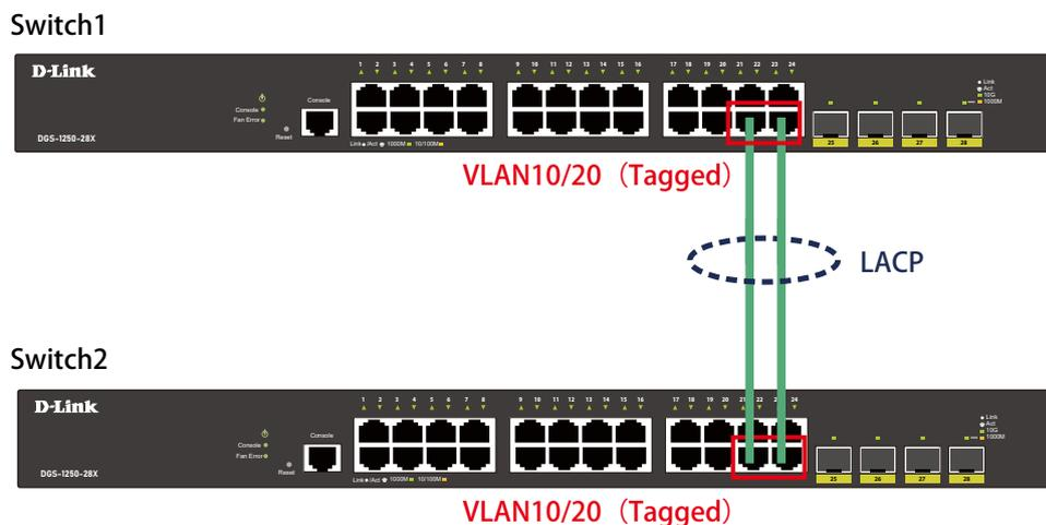
図 18-3 Link Aggregation (DGS-1250-28X)
