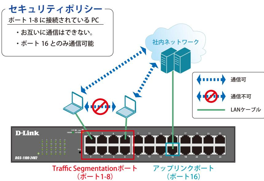
図 16-1 Traffic Segmentation (DGS-1100-24V2)
