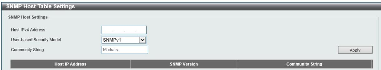
The screenshot shows the 'SNMP Host Table Settings' interface. It includes fields for 'Host IPv4 Address', 'User-based Security Model' (set to 'SNMPv1'), and 'Community String' (with a '16 chars' limit). An 'Apply' button is on the right. Below the fields is a table with columns for 'Host IP Address', 'SNMP Version', and 'Community String'.
