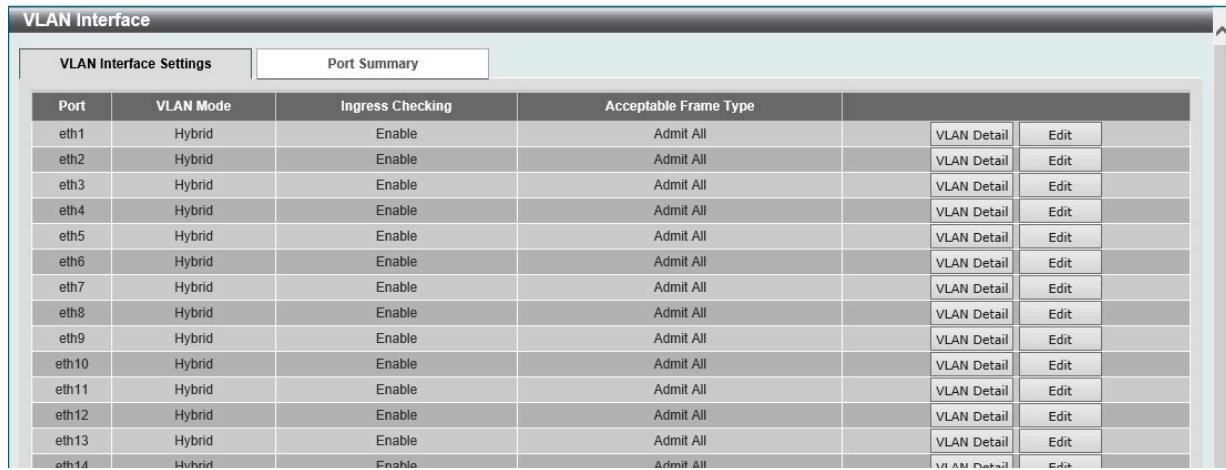
The screenshot shows a table titled 'VLAN Interface Settings' with two tabs: 'VLAN Interface Settings' and 'Port Summary'. The table has columns for Port (eth1-eth14), VLAN Mode (Hybrid), Ingress Checking (Enable), and Acceptable Frame Type (Admit All). Each row contains a 'VLAN Detail' button and an 'Edit' button.
