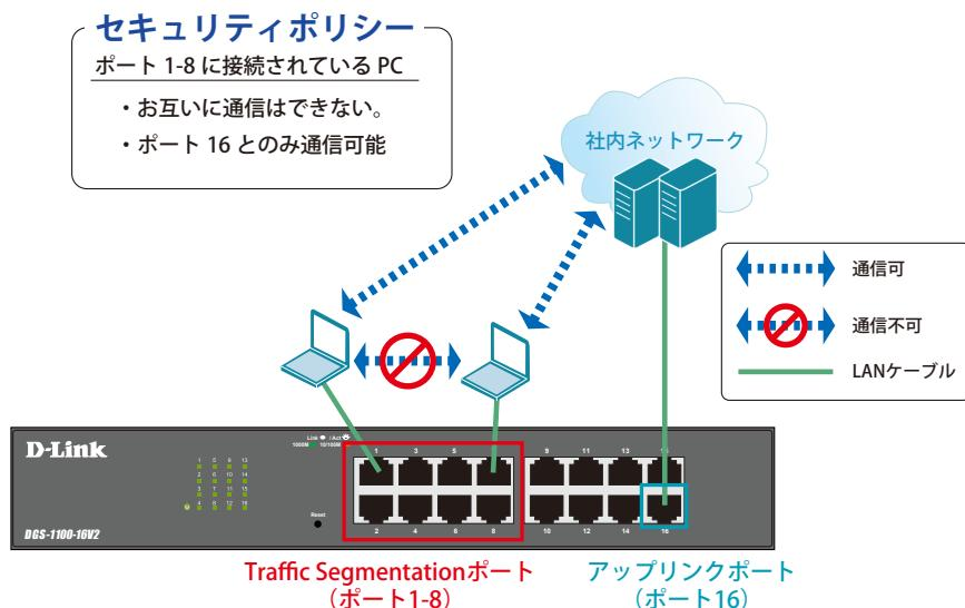
図 1-1 Traffic Segmentation (DGS-1100-16V2)
