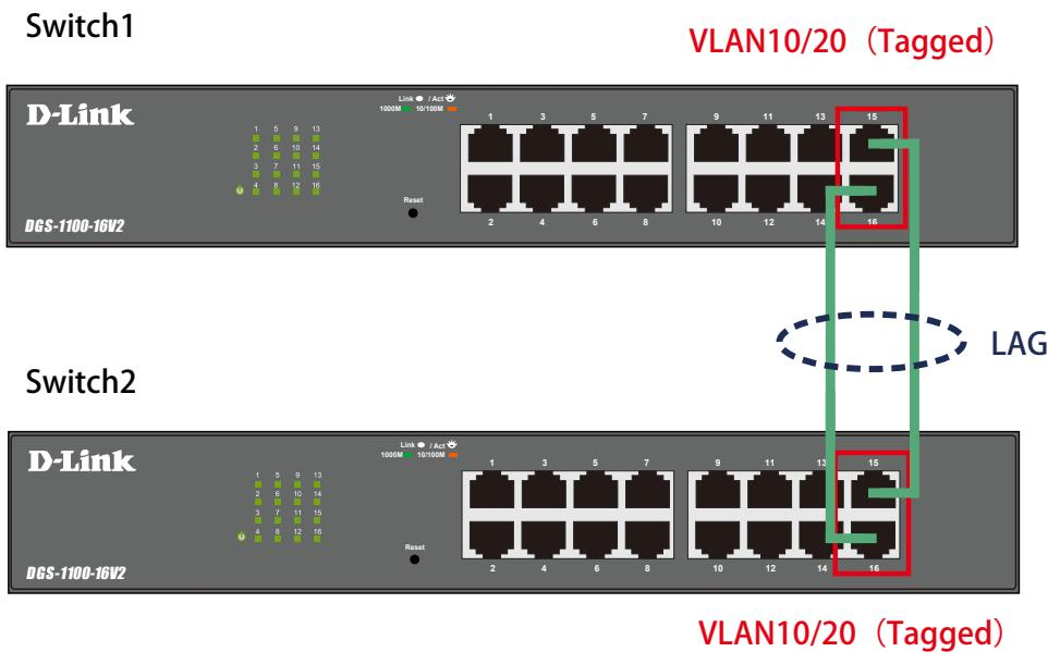
図 1-11 Link Aggregation (DGS-1100-16V2)
